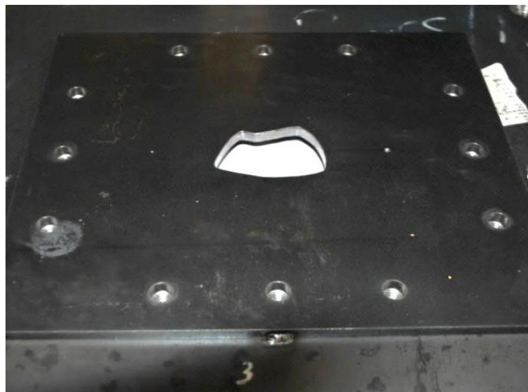
Figure 48: The backing plate with profile-specific cavity with 5mm offset
