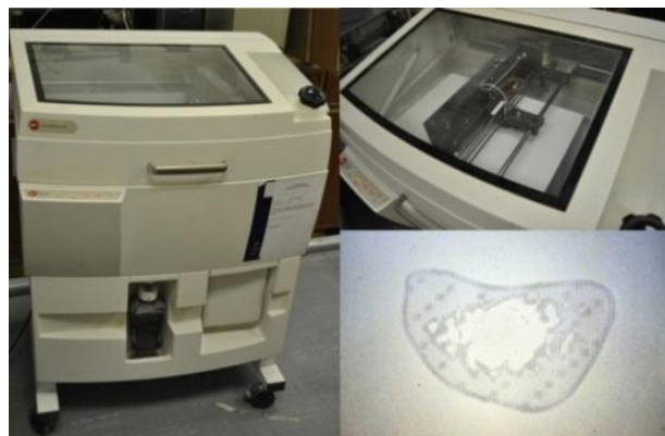
Figure 36: Z Corp 3D printer with sample profile layer
