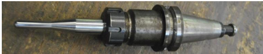
Figure 41: The forming tool installed in the chuck
