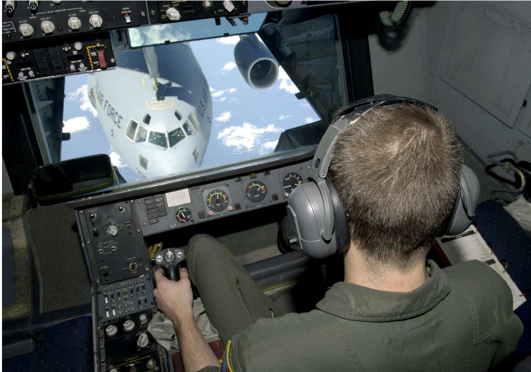
Figure 1.2: KC-135 Boomer catching the receptacle of a C-17 Globemaster.
