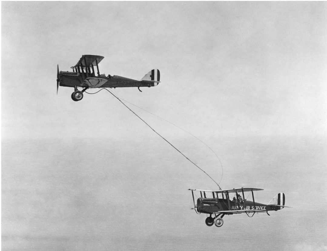
Figure 1.3: De Havilland DH-4B biplanes performing piloted aerial refuelling, using a 50 ft rubber hose and the so-called 'dangle-and-grab' refuelling system to transfer fuel from the top plane.
