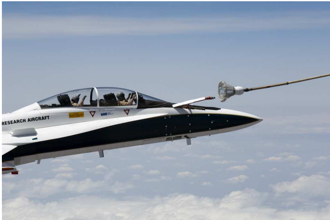
Figure 1.1: F-18 autopilot lines up the aircraft's refuelling probe with a Boeing 707 paradrogue basket.
