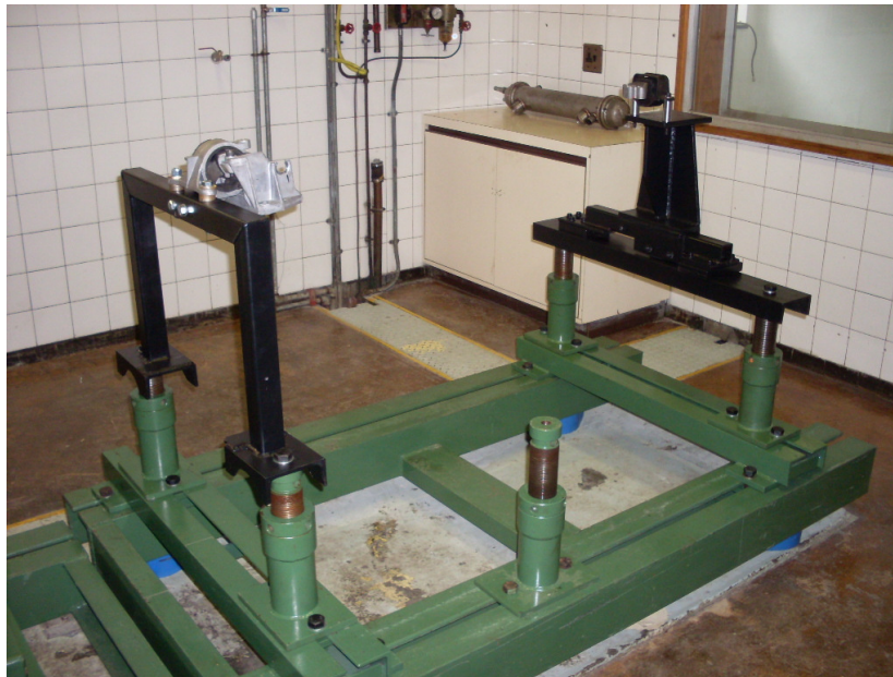
Figure 21: Test bed and engine mounting accessories
