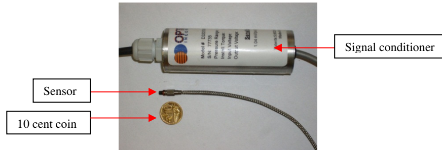
Figure 38: Optrand miniature pressure transducer
