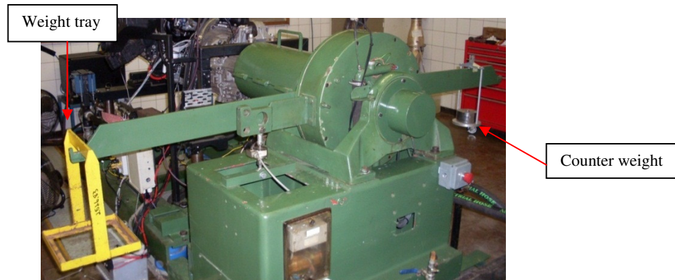
Figure 36: Load cell calibration
