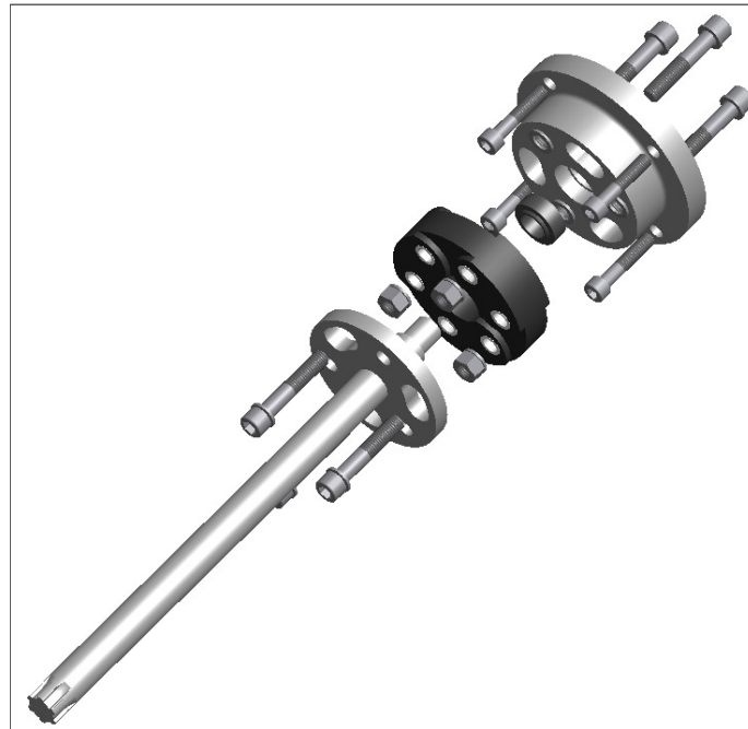
Figure 76: Drive shaft exploded CAD model
