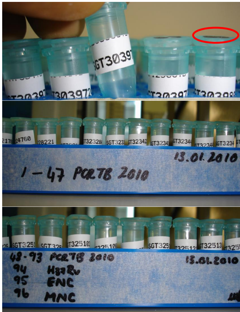
Figure 49: (A) The tube (here containing extracted DNA) will have the unique patient ID on its side and the corresponding worksheet number on its lid (circled in red). The number on the lid corresponds to the number of the screw-cap tube containing the live bacilli or patient specimen, which in turn corresponds to the number on the worksheet. (B & C) The batch number of the specimens that were extracted is written on a larger label that is taped to the side of the rack. The rack that contained the live bacilli would have had an identical label on it. The date on which the extraction was done, and the signature of the person who did the extraction must be on the label. The Extraction positive control (H37Rv) and the Extraction negative control (ENC) are numbers 94 and 95 respectively. Tube number 96 acts as place holder for the master mix negative control (MNC). Please note that the unique patient identifier numbers in example (A) consists of 8 digits (SGT 30397***), and the specimens are not to be confused as all being SGT30397.
