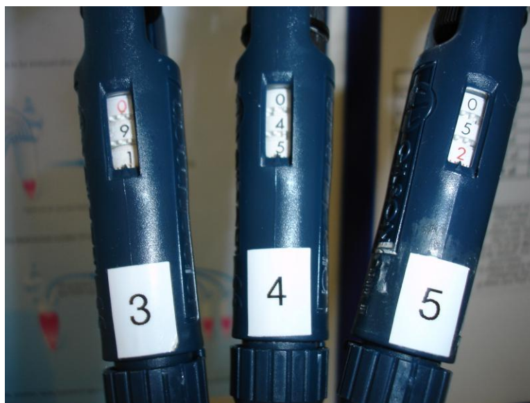
Figure 33: Area specific numbering of the pipettes. Shown here are the pipettes that are used in the reagent preparation area.
