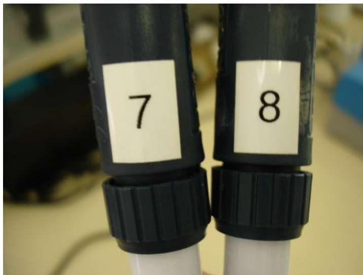
Figure 39: Area specific numbering of the pipettes. Shown here are the pipettes that are used in the hybridization area.
