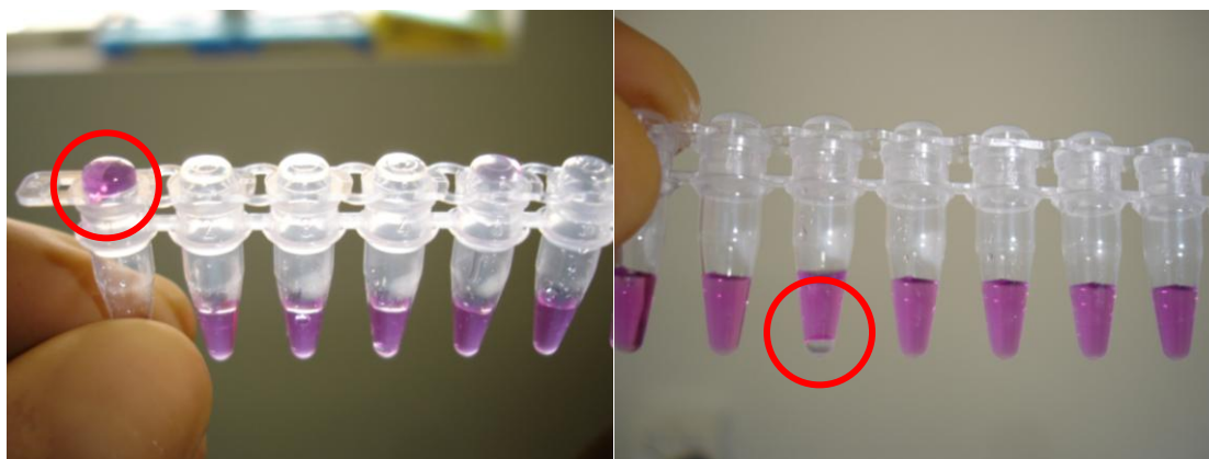
Figure 56: Examples of what to look for during visual inspection of the PCR reaction tubes before they are placed in the thermal cycler. (A) No liquid should be in the domed-caps. If seen, the tubes can be briefly spun down in a mini-fuge or swung down by hand. (B) All bubbles at the bottom of the PCR reaction tubes must be cleared by lightly tapping the bottom of the tubes on the bench (without getting any of the liquid in the lid), or spinning in a mini-fuge.
