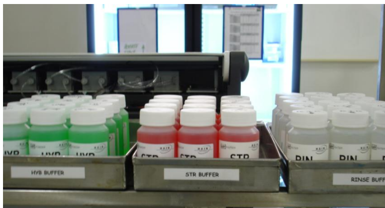
Figure 43: Ambient temperature storage of the HYB and STR buffers (requiring pre-heating before the hybridization process) and the RIN buffer. The lids are dated to ensure the reagents are not outdated and are used in the order received.
