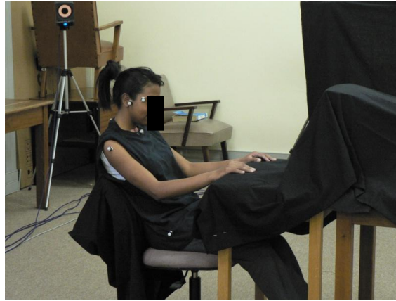
Figure 4.6: The placement of the reflective markers for validity testing
