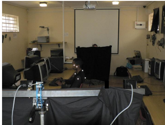
Figure 4.9: 3D-PAT set-up in the school computer classroom, showing the placement of the cameras in relation to the student
