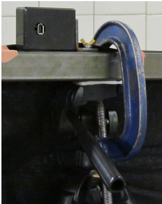
Figure 3.1(b): A close-up photograph of the camera unit, showing a centre camera, with the steel clamp keeping the cross-bar firmly on the tripod
