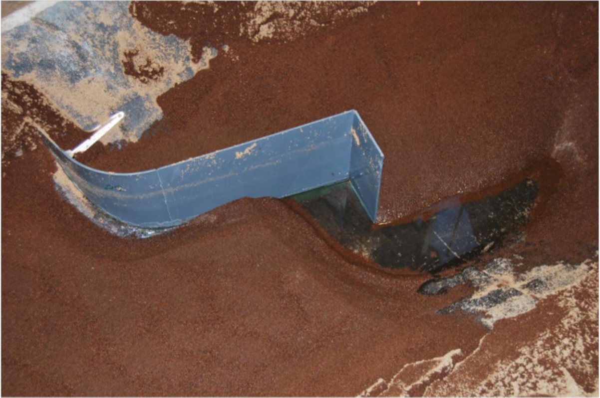
Figure A-17: Photo 3 of 30° structure with L-shaped attachment
