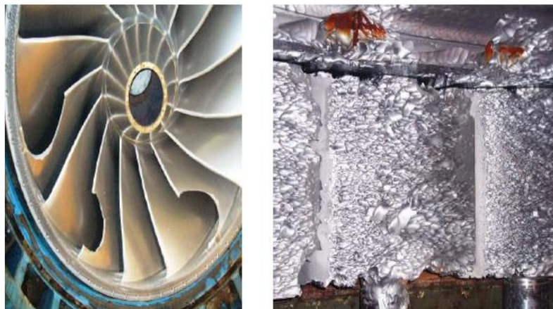
Figure 1.1: Eroded runner and guide vanes (Olesen and Pradhan, 2010)
