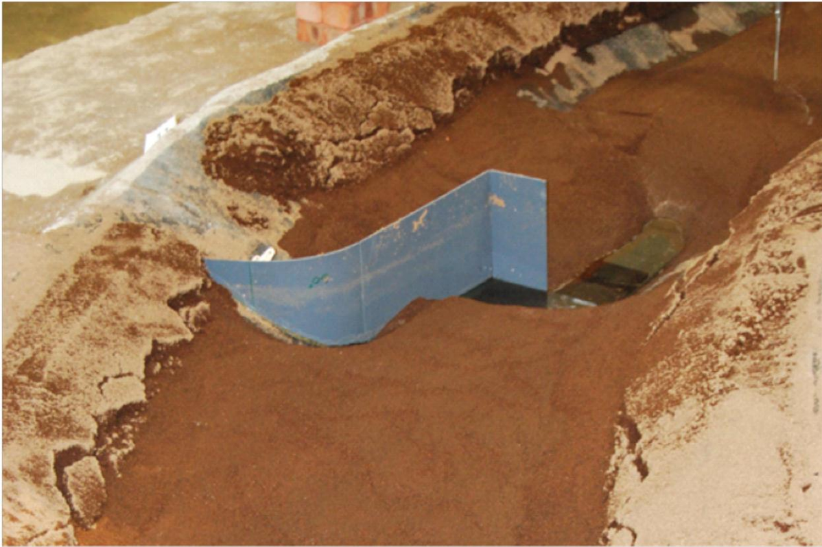
Figure A-15: Photo 1 of 30° structure with L-shaped attachment
