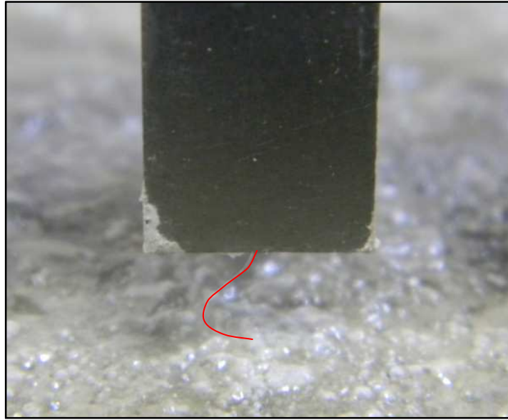
Figure 3.15: Curved fibre before pullout, with the fibre indicated in red
