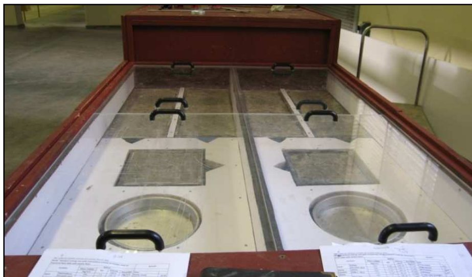
Figure 3.3: Test compartment with Perspex covers and PVC lining inside
