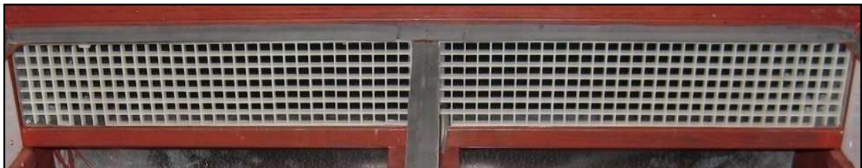
Figure A3: Plastic screen used at the beginning of the test compartment
