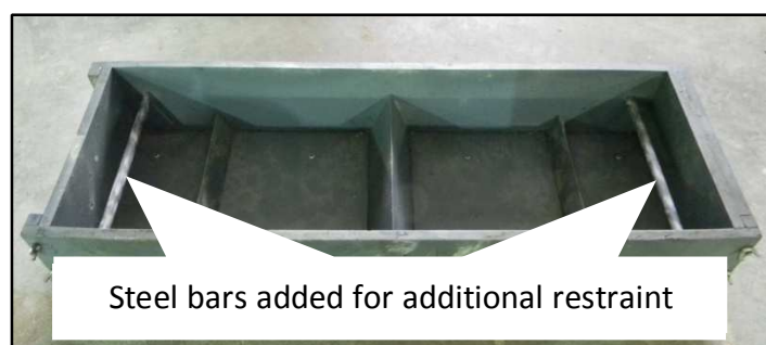
Figure 4.1: PSC mould with steel bars for additional restraint
