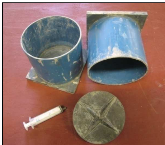
Figure 3.10: Bleeding moulds, syringe and device used to create tracks
