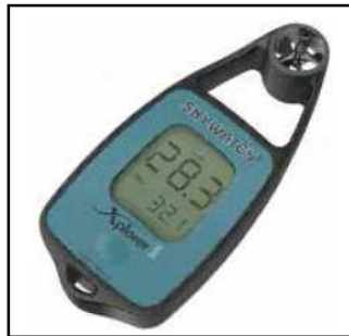
Figure 3.4: Hand held anemometer for wind speed measurements
