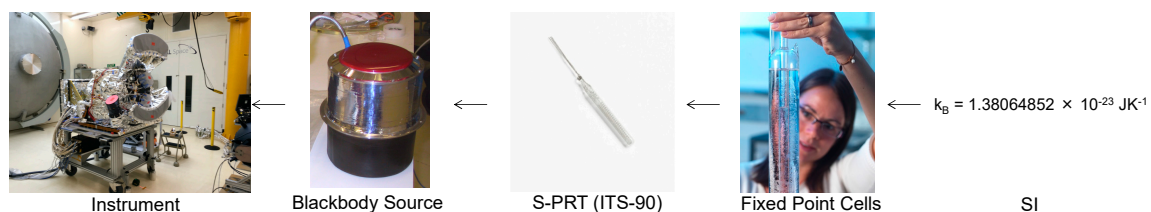
Figure 1. Illustrating the traceability of the SLSTR radiometric calibration via blackbody sources to ITS-90.
