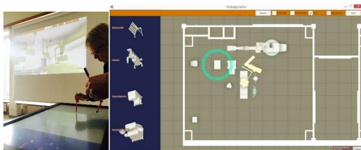
234 235 Fig. 2. Left: The multi-touch table used together with a non-immersive VR display. Right: The layout of the multi-touch table 236 screen. Available components are accessible from a scrollable panel on the left side and are added to the scene using drag- 237 and-drop.
