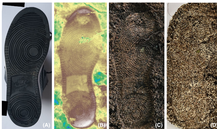
FIGURE 2 Aligned images before grid overlayed and features recorded. (A) Rectified image of Nike 2 (hightop trainer) sole. (B) 2D render from DigTrace of impression made from Nike 2. (C) 2D image of impression made from Nike 2. (D) Cast made from impression, made from Nike 2
