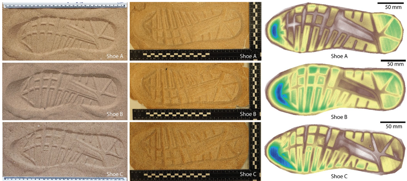
FIGURE 5 Left column shows vertical photographs of impressions made in sand with artificially damaged shoes (A), (B, and (C). Middle column shows a set of photographs of castings output made from left impressions. Right column shows SfM photogrammetry outputs from left hand impressions. 3D point clouds have been interpolated and rendered in 2D 'terrain'. Multiple color renders available, each bringing out different elements of detail. Shoe (A) Low-level damage output. Shoe (B) Medium level damage output. Shoe (C) High-level damage output
