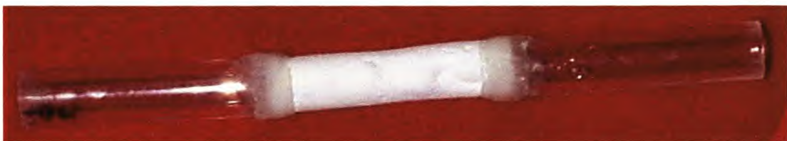
Figure 5.2: Picture of the tested membrane mounted between 2 perspex tubes
