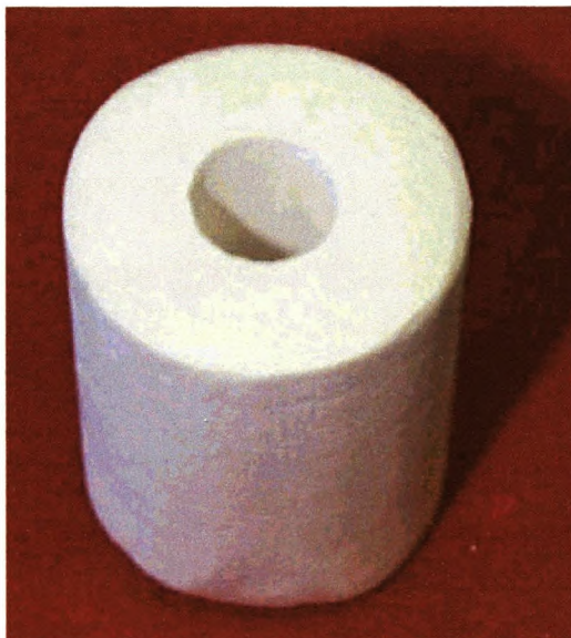
Figure 4.4: Drawing and picture of a typical gypsum mould
