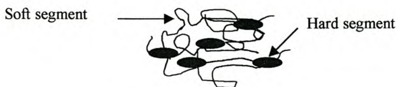
Figure 2.6 Schematic representation of the domain structure in segmented polyurethanes
