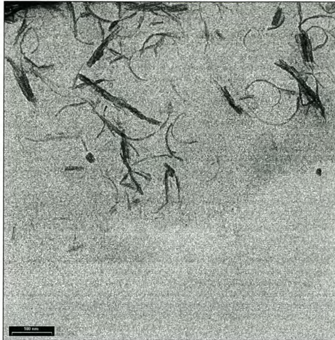
Figure 6.3-13 Bent fibrillar particle shapes from 16.9 % cross-linked guest polymer.
