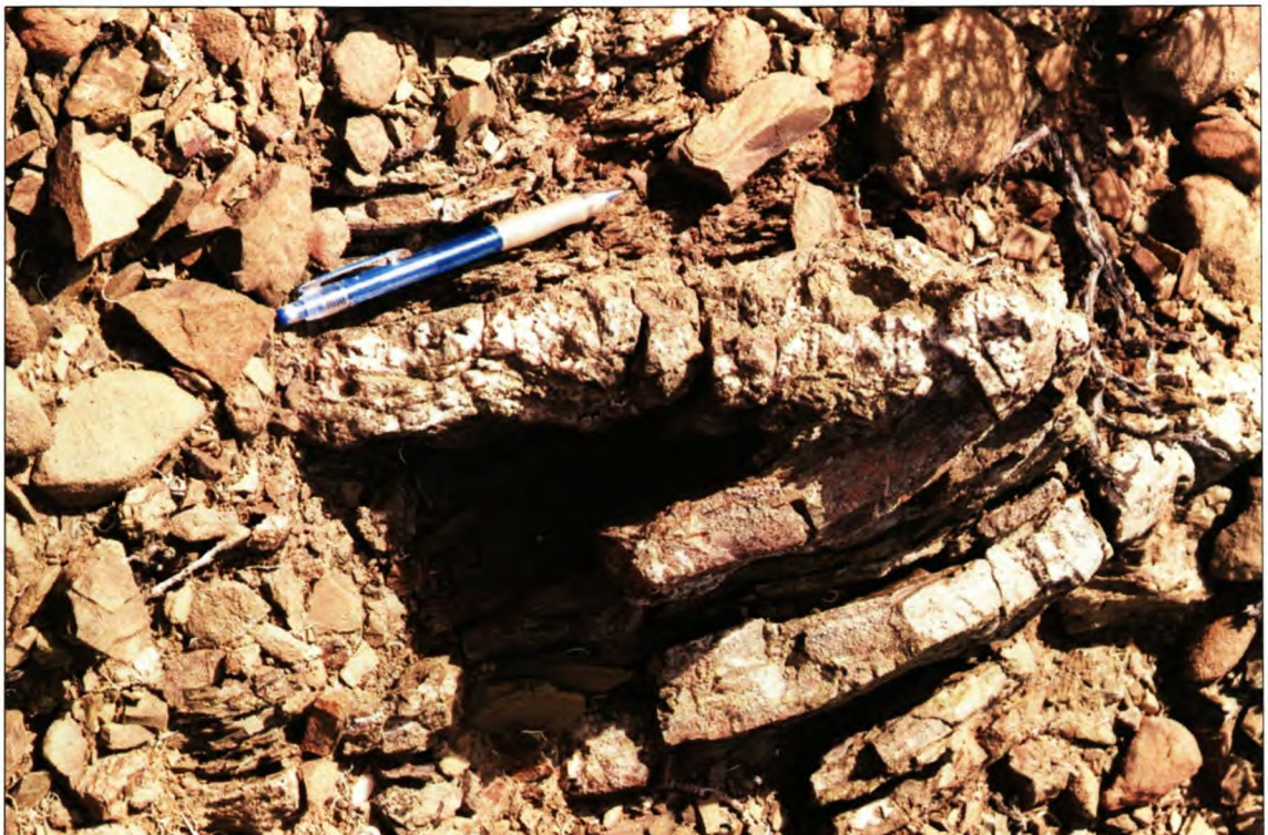
Figure 2.4.2 Breccia containing secondary quartz and calcite. Miniature overfold associated within the thrust-plane in Figure 2.4.1 (from Van der Merwe, 2003).
