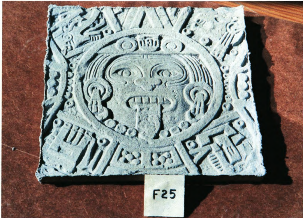
Figure 3.31. Embossed Perlite panel
