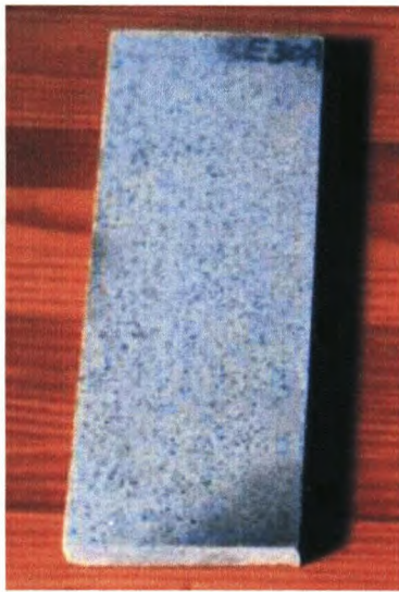
Autoclaved (oven=40°C; mc to autoclave=20%)
