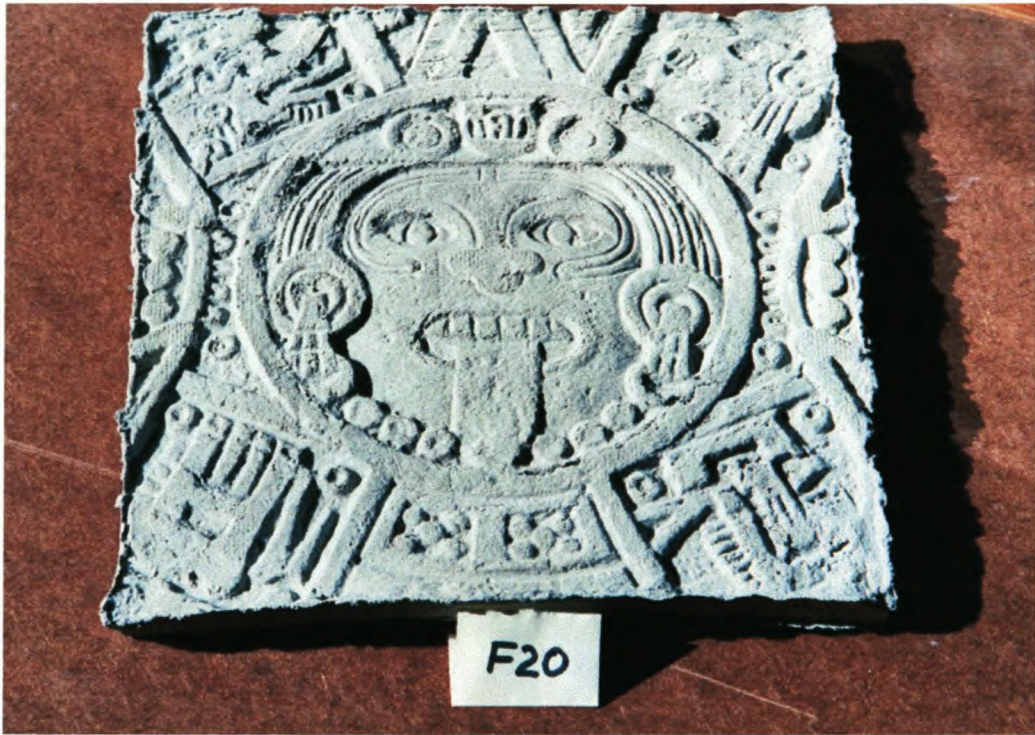
Figure 3.30. Embossed standard panel
