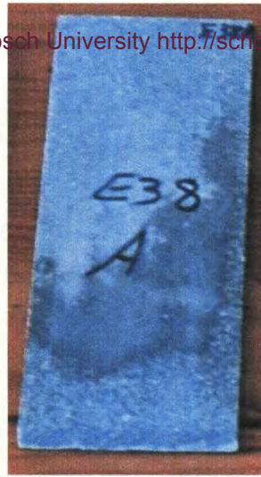
Autoclaved (oven=50°C; mc to autoclave=25%)
