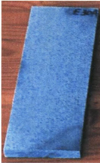
Autoclaved (oven=40°C; mc to autoclave=20%)
