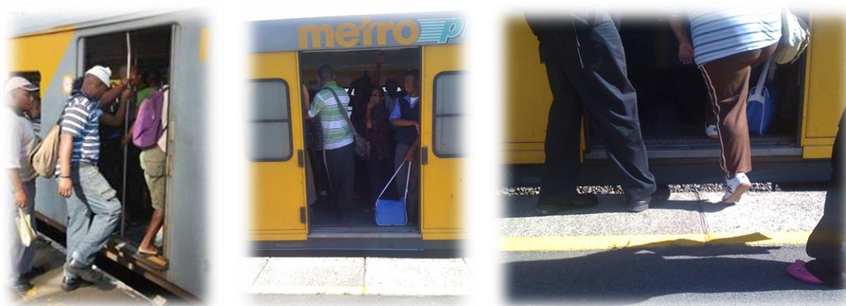
Figure 4.71: Photographs showing vertical and horizontal platform clearances
