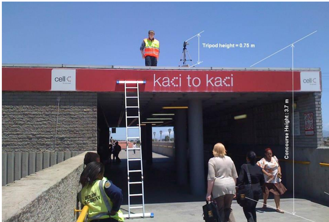
Photograph showing concourse camera placement above Measurement Area "A" at Bonteheuwel station
