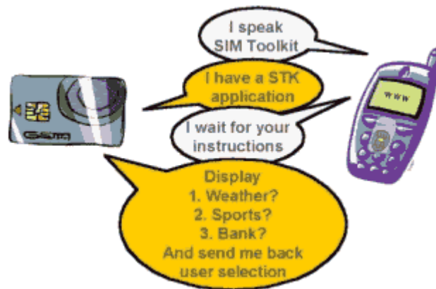
Figure 3.1: SIM Toolkit Application interaction with a cellular handset [30]
