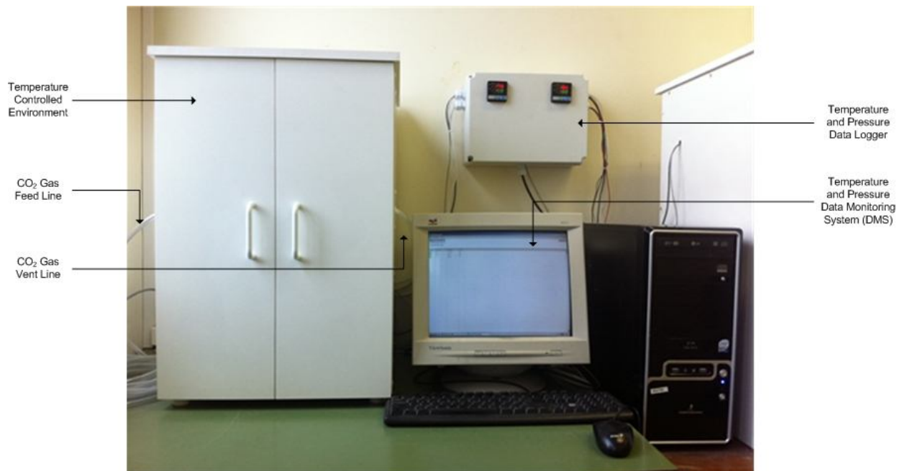
Figure 4.2 – Experimental setup with descriptions.
