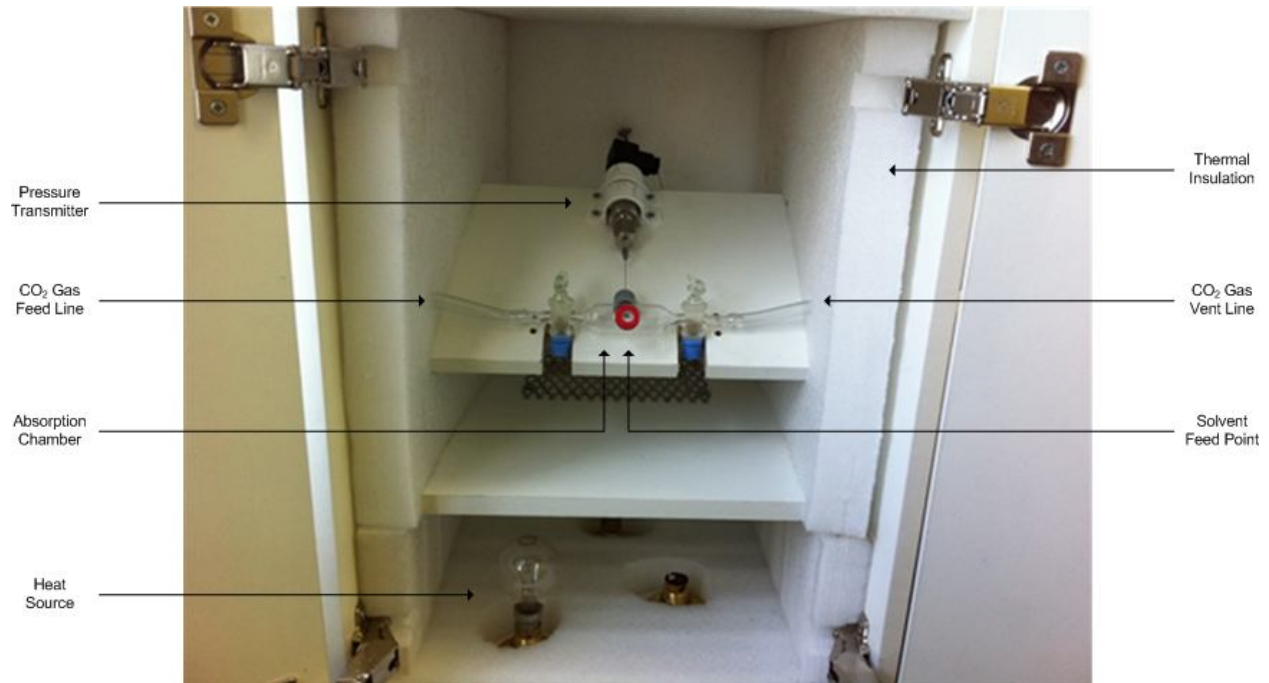
Figure 4.3 – Temperature-controlled environment of the experimental setup with descriptions.
