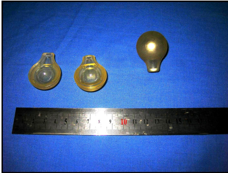
Figure 4.3: Prototype of Internal Magnet Housing
