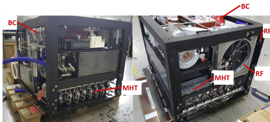
Fig. 8 – MH tank installed in the forklift power module.
