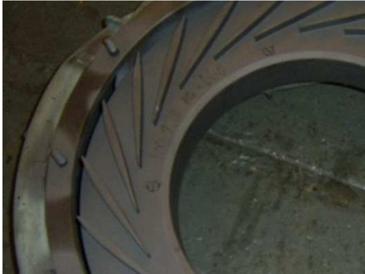
Figure 2.3: GE 7S1408 A1 compressor diffuser (Courtesy of Johan van der Spuy).
