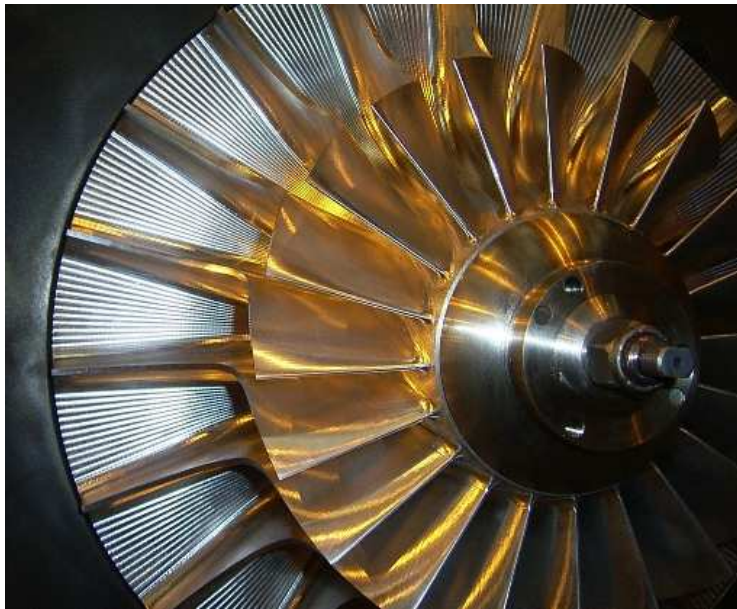
Figure 2.2: GE 7S1408 A1 compressor impeller (Courtesy of Johan van der Spuy).
