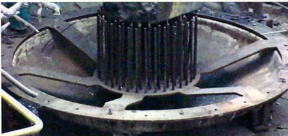
Figure 2.12: Base plate and pin arrangement of an anode of an old pilot plant DC plasma arc furnace (Mintek, 2000)
