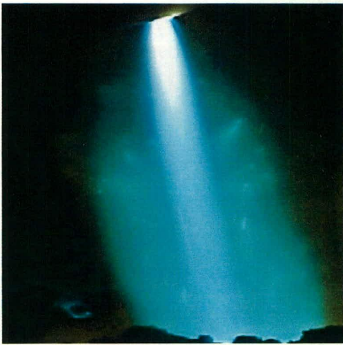
Figure 2.13: Low Current Arc, Visible core
