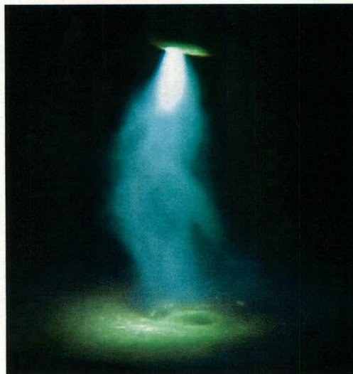
Figure 2.17: High current, diffuse arc
