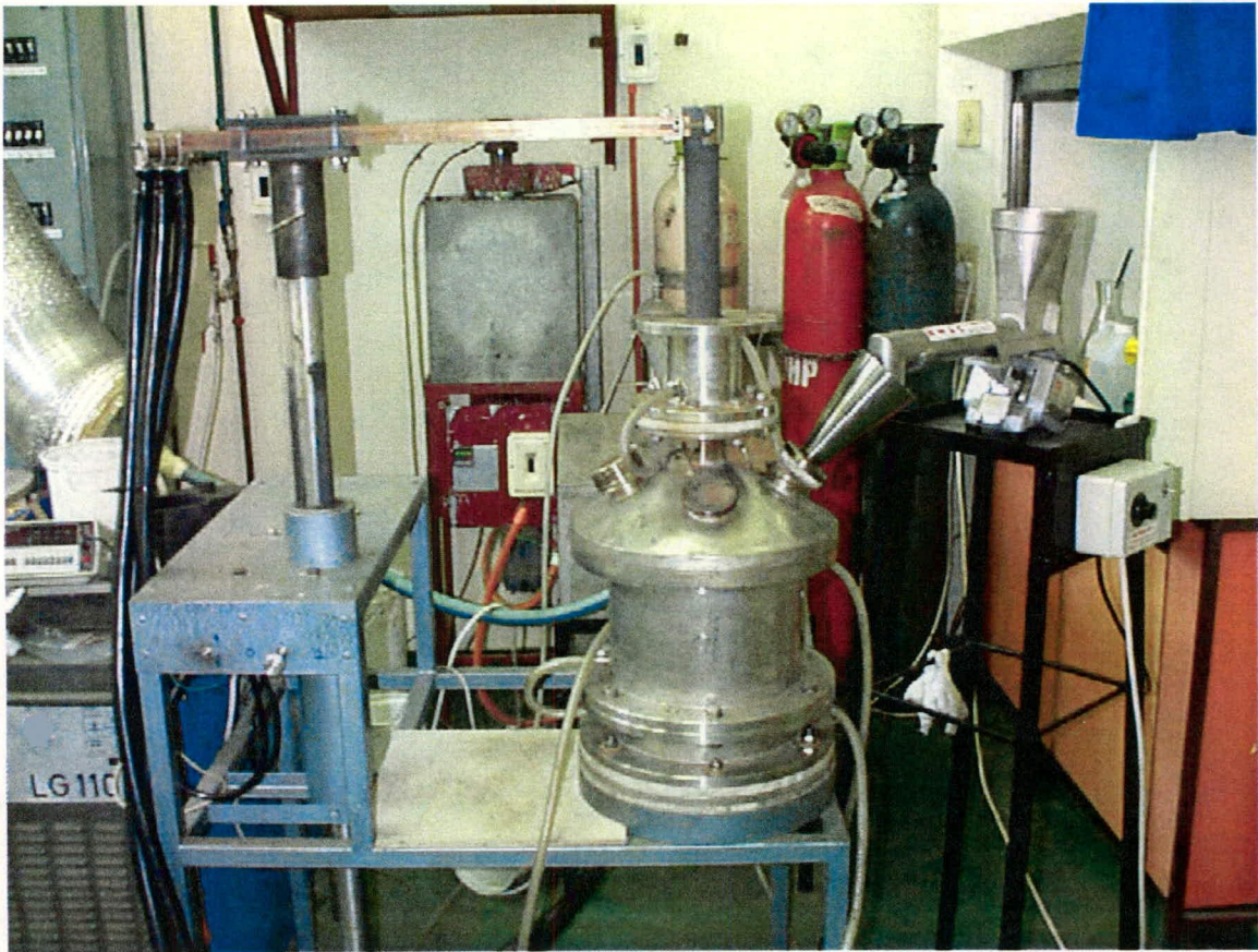
Figure 11.1: Laboratory plasma arc furnace
