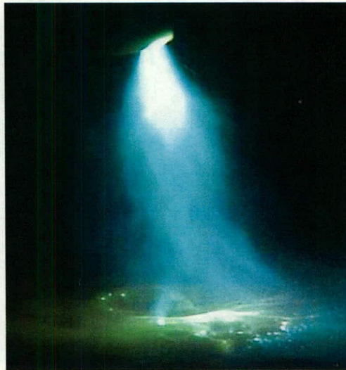
Figure 2.18: High current, diffuse arc (dimple)
