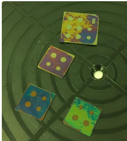
Figure 4-2: 4H-SiC PiN diodes after thermal oxidation process. The variation in colour is due to surface contamination.
