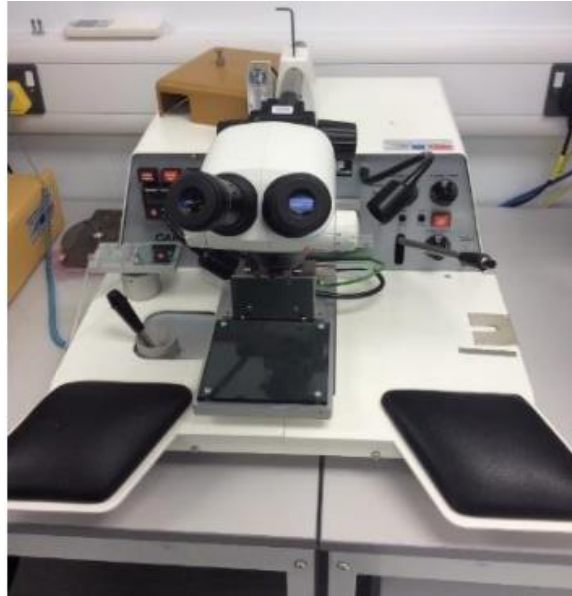
Figure 4-9: Cammax Precima EDB65 Eutetic pick and place die bonder, including N 2 cover gas at the University of Warwick power device packaging facility
