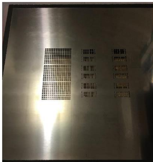
Figure 4-7: Al stencil used for soldering process with a thickness of 6 thou
