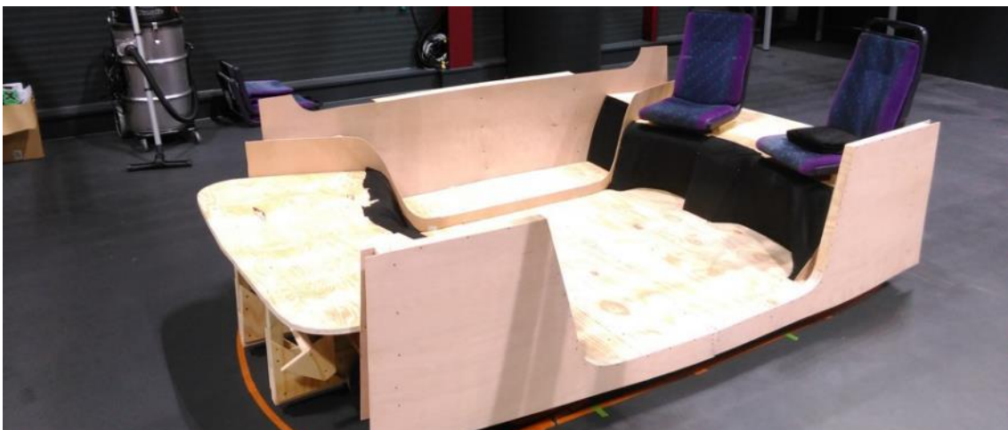
Figure 11.2 Lower Section of the Ergonomic Buck
