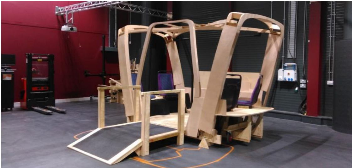
Figure 11.4 Ergonomic Buck set up for the initial trial including a placeholder ramp
