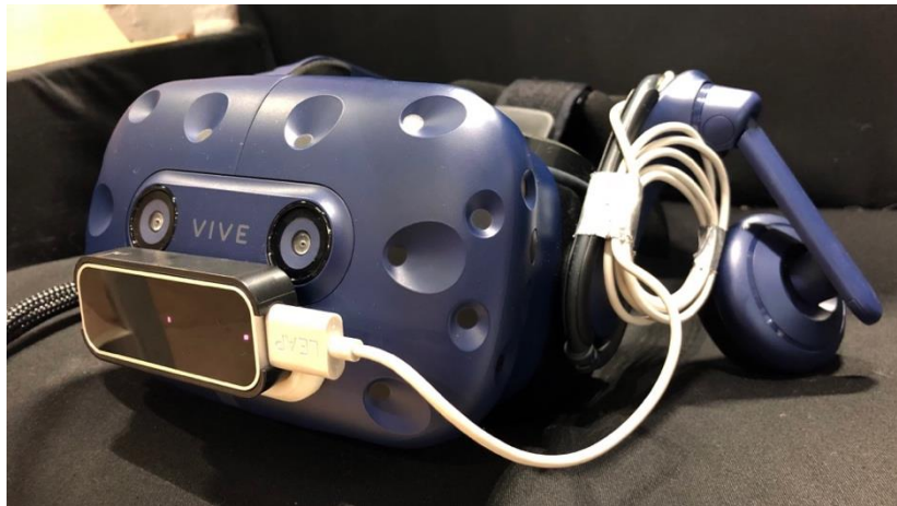
Figure 13.4 HTC Vive Pro with the Leap Motion sensor mounted
