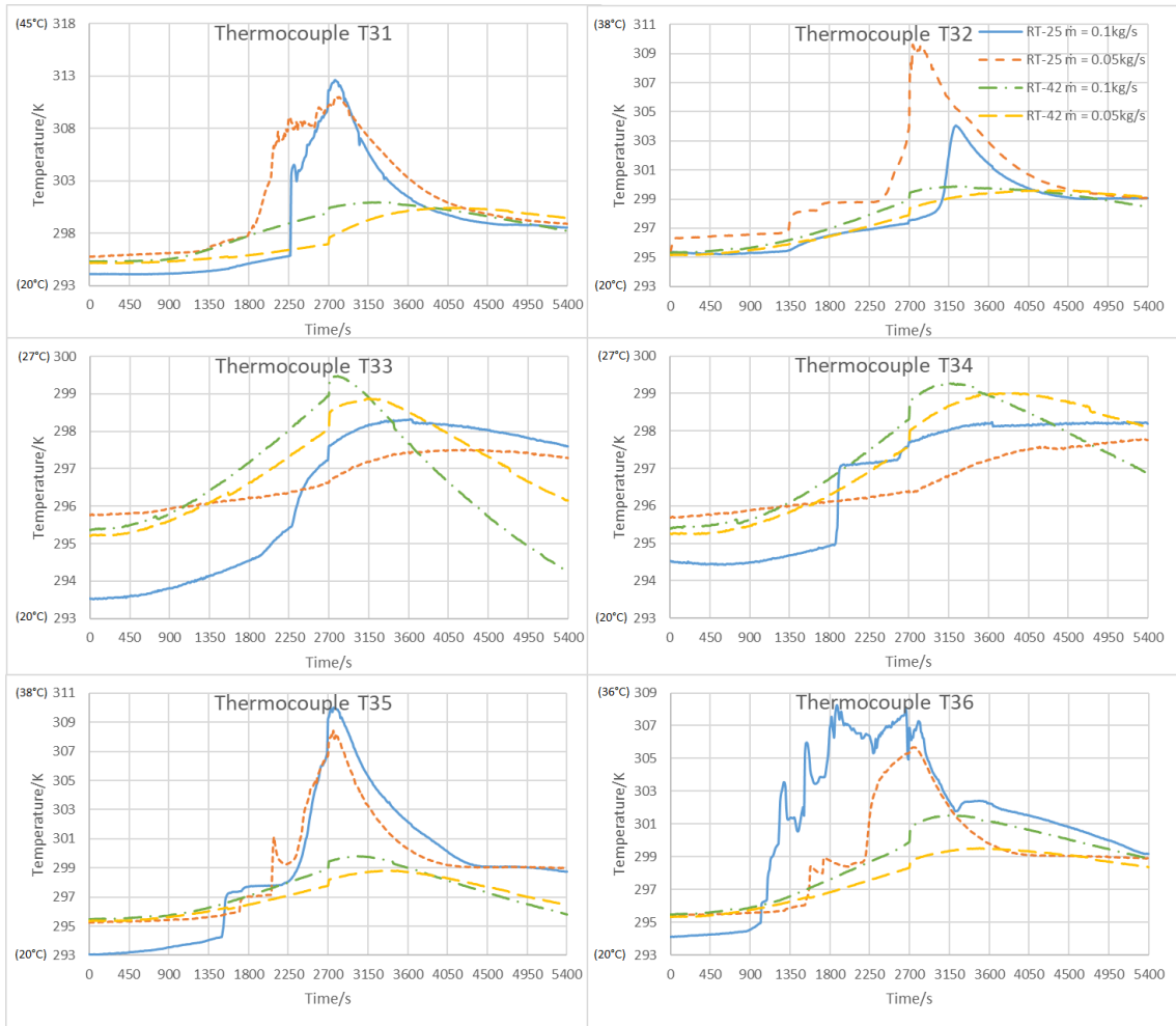
Figure B-3: Temperature variations for the upper tier of thermocouples in the solo-flow strategy
