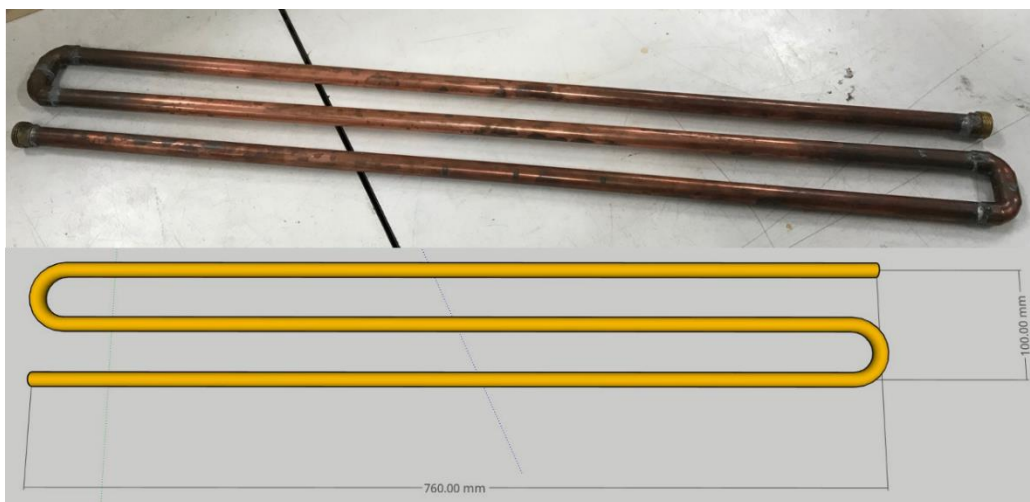
Figure 5-4: Layout of the copper pipe of the GW and CW flows with a 12.7mm diameter
