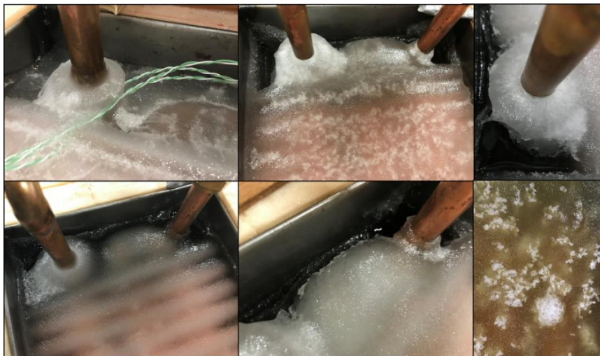
Figure 5-19: Shrinkage of volume and air bubble formation, due to ullage after the freezing of the PCM
