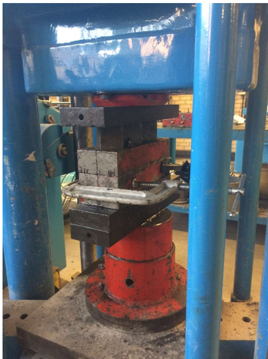
Figure 5.7: Gang of three 50mm mould compacted at 90KN
