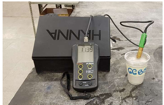
Figure 4.8: Saturated Samples ready to be Tested and Hanna Instrument
