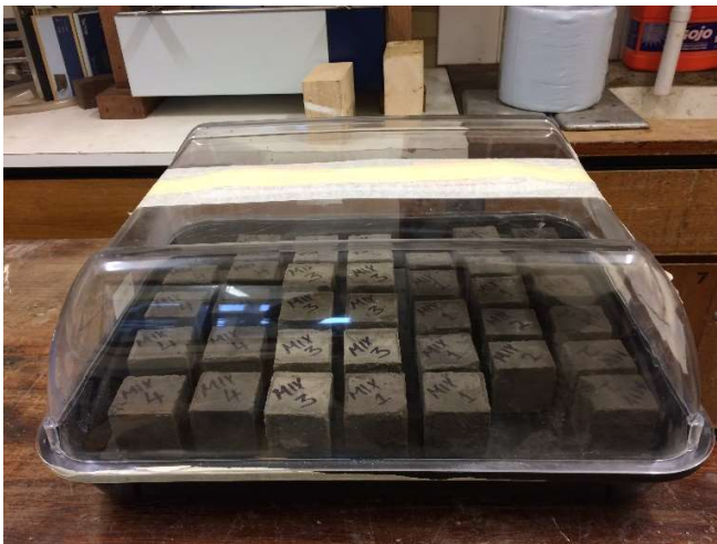
Figure 5.9: Specimens being cured in propagator
