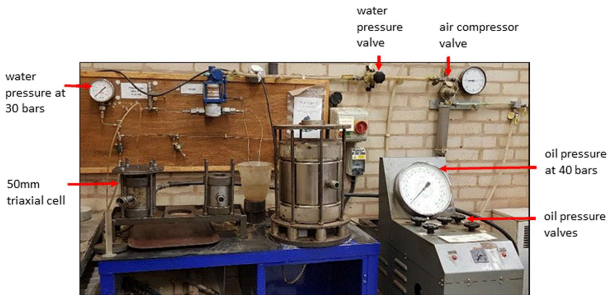
Figure 8.1: High Pressure Flow Test Layout
