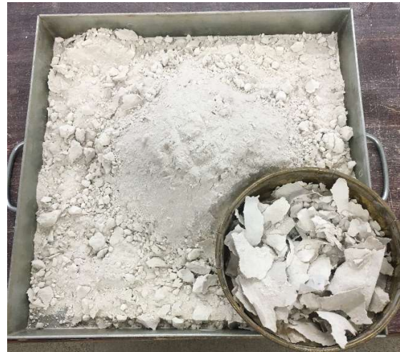
Figure 5.3: Sieving of plasterboard to remove paper
