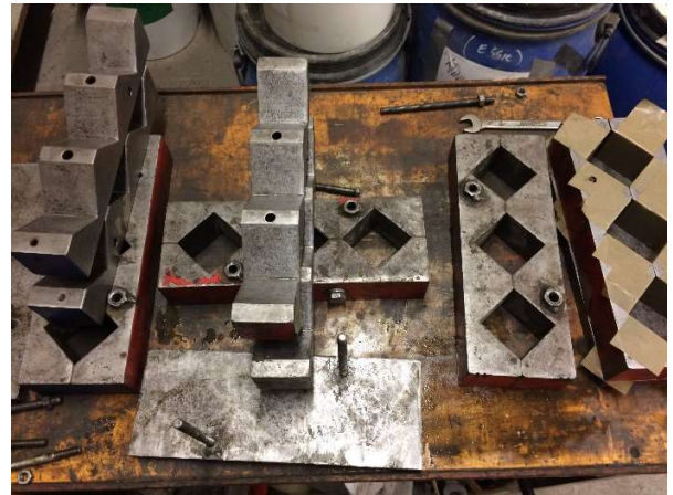
Figure 5.6: Gang of three 50mm cube moulds being prepared for use
