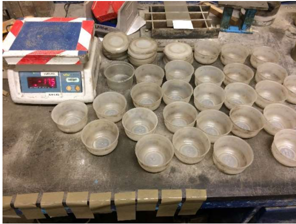
Figure 5.5: Weighing scale and plastic containers used to place 90g sample
