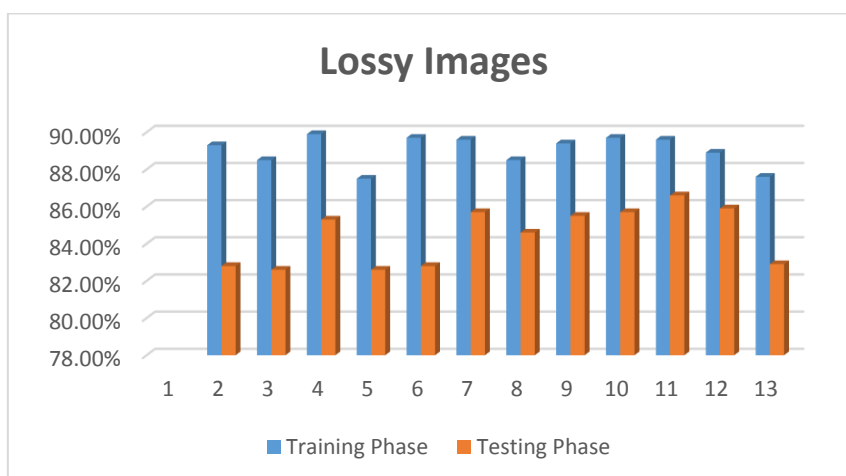
Figure 5.12: Representation of the Accuracy Rates during the Validation Process for the Lossy Images using MLP.
