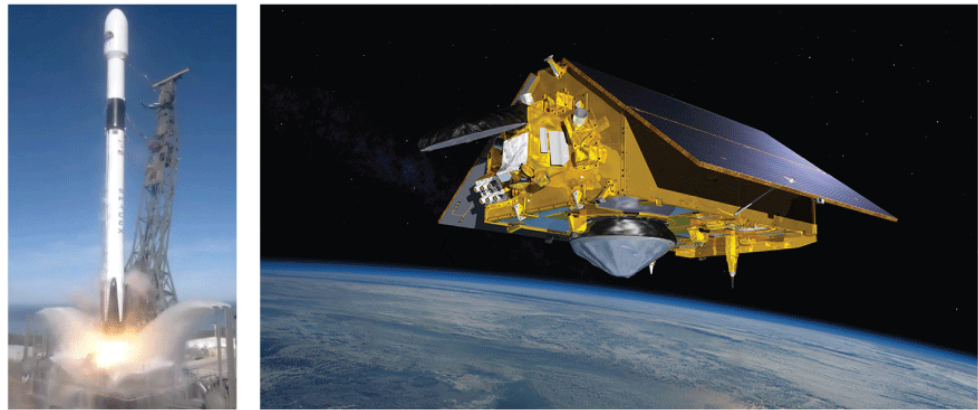
Figure 2. Sentinel-6 Michael Freilich was launched on 21 November 2020 and will be the first to offer fully focused SAR operation over all the ocean between 66°S and 66°N. To achieve a precise intercalibration it will be in a tandem orbit within 30 s of Jason-3 for 12 months. Images courtesy of NASA and ESA.
