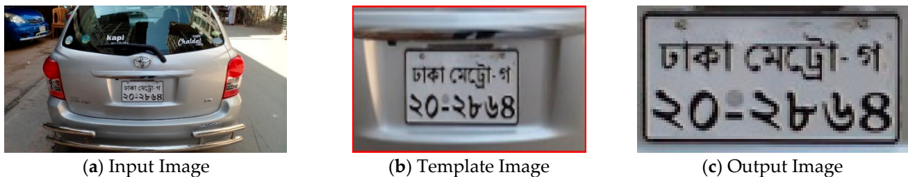
Figure 6. Localization of the number plate region by using the template matching technique: (a) input image; (b) template image; and (c) output image.
