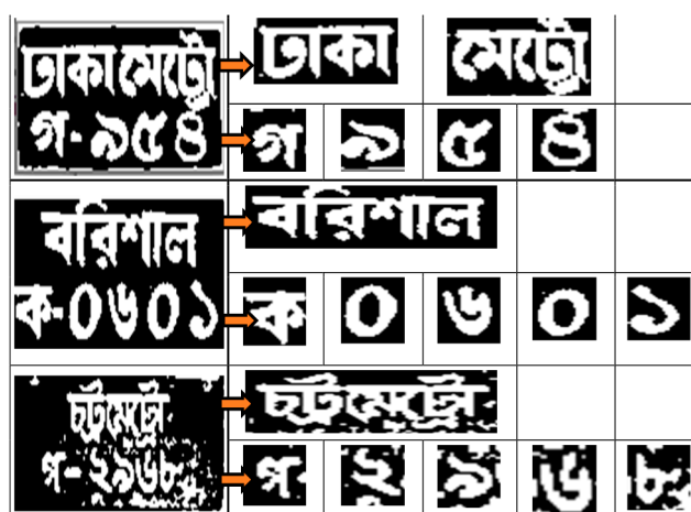
Figure 9. Segmentation performed of each part of three different number plates.
