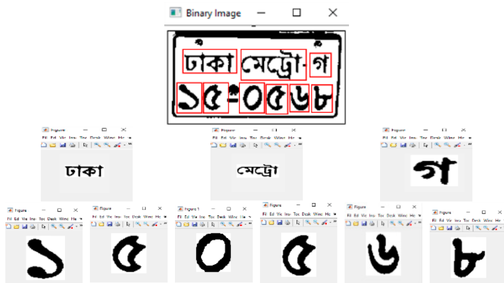
Figure 12. Example of character segmentation from a vehicle number plate.
