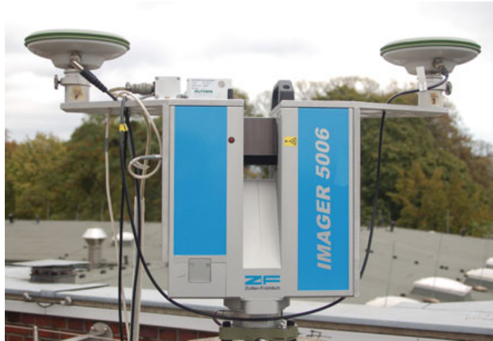
Fig. 1 Prototypical realization of the MSS formed by a laser scanner (blue) and two eccentrically mounted GNSS antennas (green). This MSS was used for the field experiment
