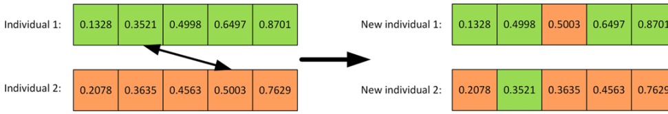
Figure 3: Example for random pointwise crossover: Both individuals consist of n - p = 5 internal knots. In individual 1 the second internal knot and in individual 2 the fourth internal knot is chosen randomly. These knots are exchanged between the individuals and subsequently each individual has to be assorted.
