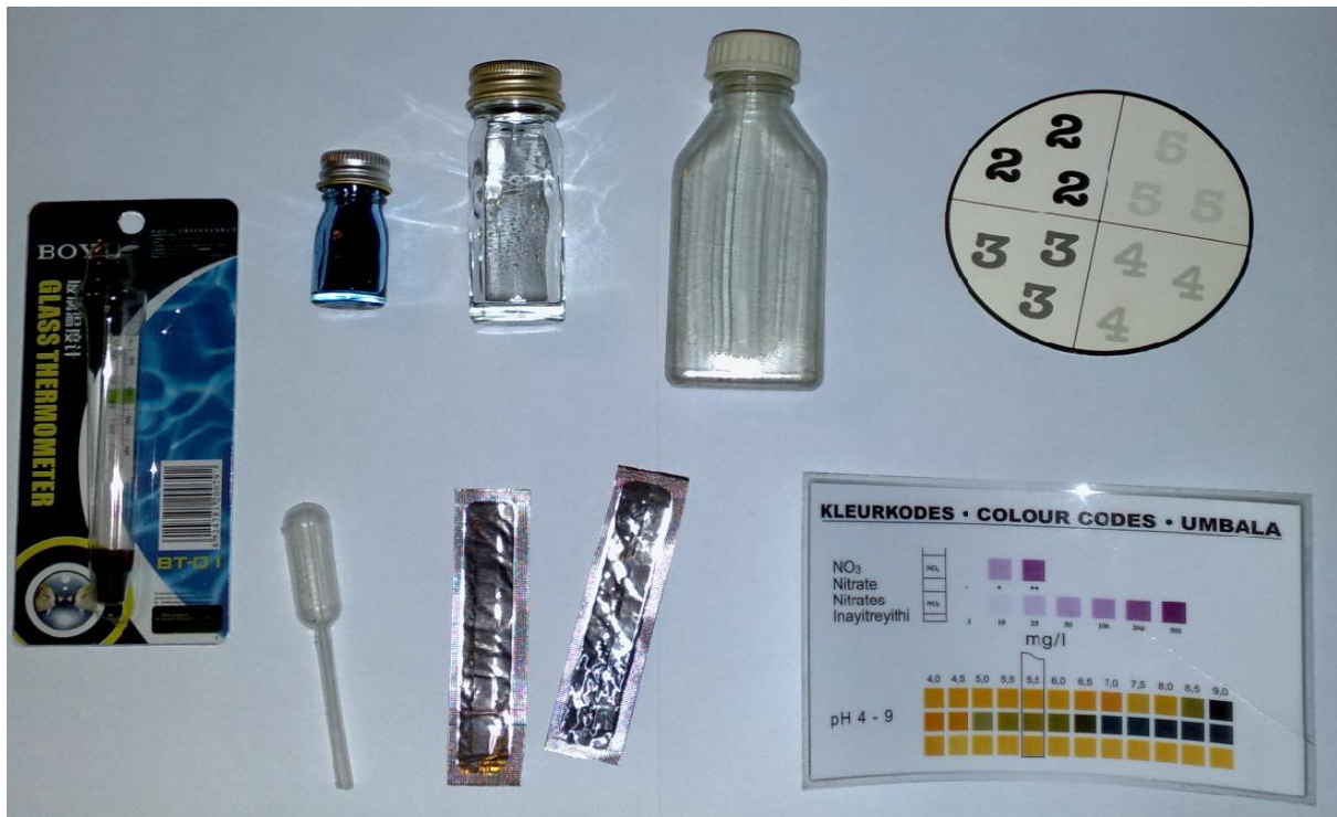
Figure 17: The water-testing kit that was used for empirical data collection.
