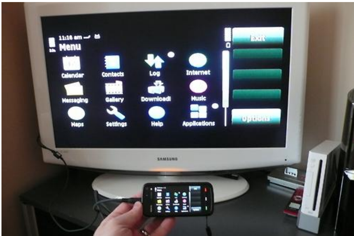
Figure 2: Mobile devices are able to be connected to external displays such as monitors and data projectors, enabling them to play the roles of the desktop computers or laptops that are otherwise connected to these displays.
