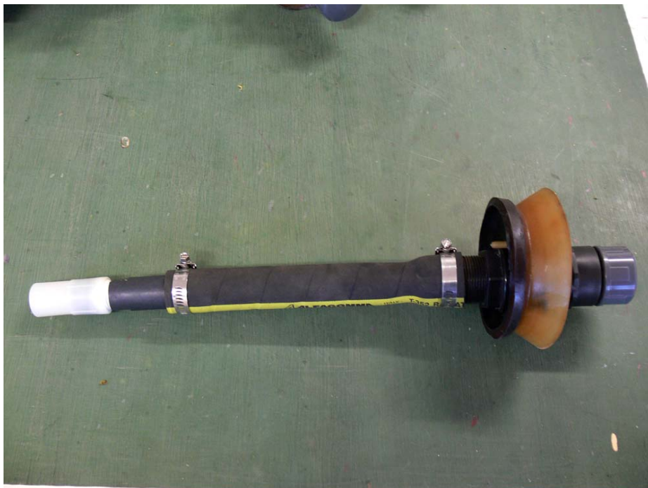
Figure 3.3 The TruTrack Data Logger (Model pH-HR mark 4, Intech Instruments LTD, NZ) used for rumen pH logging, inside cannula plug mounting ready for insertion into the rumen of cannulated cow
