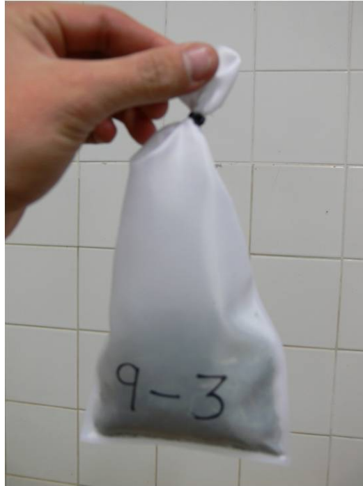
Figure 3.7 A dacron bag, labeled with a material marker, filled with five gram of kikuyu/ryegrass pasture and sealed with a cable tie, ready for insertion into stocking
