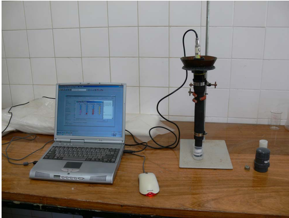
Figure 3.2 TruTrack Data Loggers (Model pH-HR mark 4, Intech Instruments LTD, NZ) connected to a laptop for logger calibration and data downloading with the Omnilog Data Management Program Version 1.64
