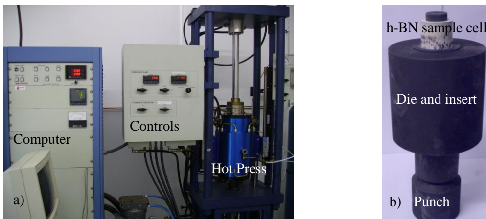
Figure 5.37: The equipment for the diffusion experiment: a) The Uni-axial hot press and b) the hot-zone components
