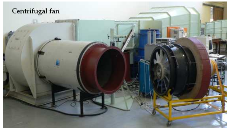
Figure 3.4 Picture of the multiple turbine rig and the wind tunnel (detached to show the turbine rotor).
