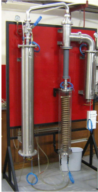
Figure 8: Heat-driven refrigeration test unit 20
