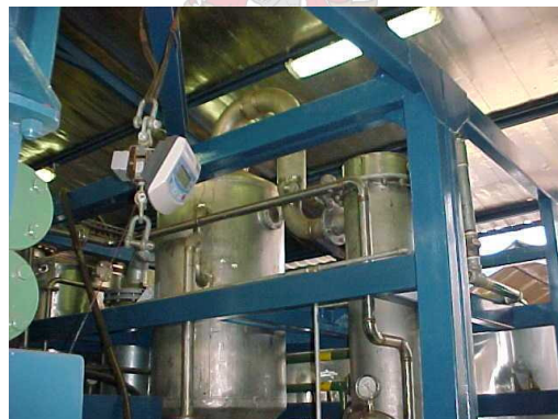
Figure 4.8: The vapour-liquid separator and condenser.
