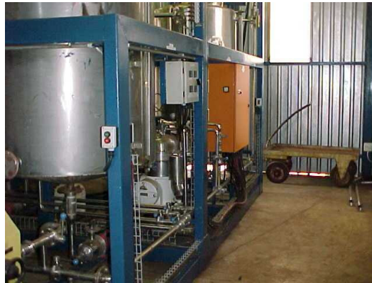
Figure 4.7: Skid 1, with the dilution tank in the back, and only a corner of the filter showing.
