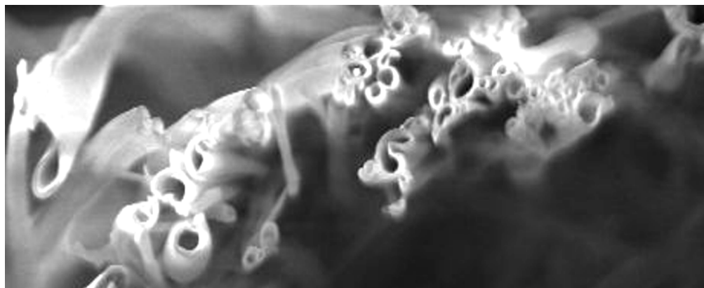
Figure 4.7: SEM image of hollow fibers electrospun from a 12 wt % CA solution. Mag (877x)
