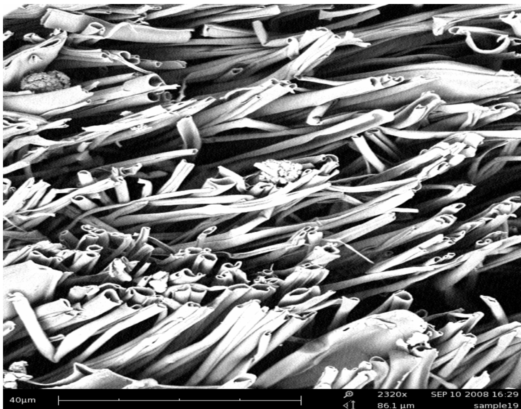
Figure 4.15: SEM image of electrospun hollow fibers produced using a CA polymer concentration of 14 wt % at a distance of 8 cm.
