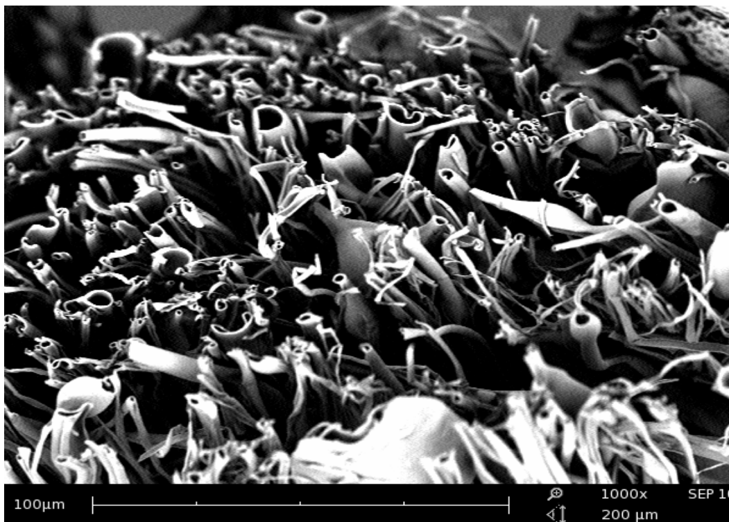
Figure 4.14: SEM image of electrospun hollow fibers produced using a CA polymer concentration of 14 wt % at a distance of 11 cm.
