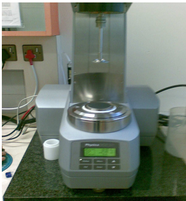
Figure 3.3: Picture of Paar Physica MCR 501 modular compact rheometer used to measure the viscosity of polymer solutions.
