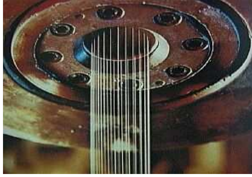
Figure 2.1: Fibers produced from a melt spinning machine [7].
