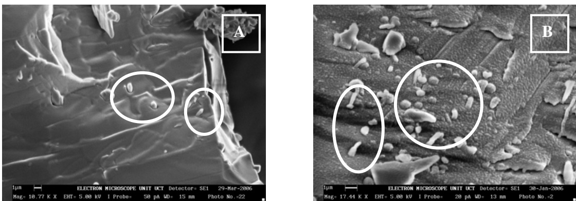
Fig. 4.18: Microtubes from OL1 [A] and OL2 assemblies [[B] after 15 days in 0.1% TEA.
