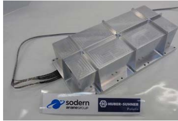
Fig. 8 Picture of the OPTIMA 48-port switch breadboard
