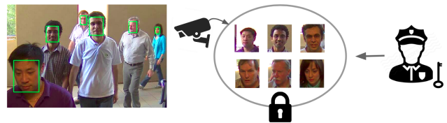
Figure 1: Overview of our proposed approach. For each subject, we automatically extract one high quality frame (or face crop) and encrypt it for storage. Access to the images is only possible after legal authorization in case of an investigation.
