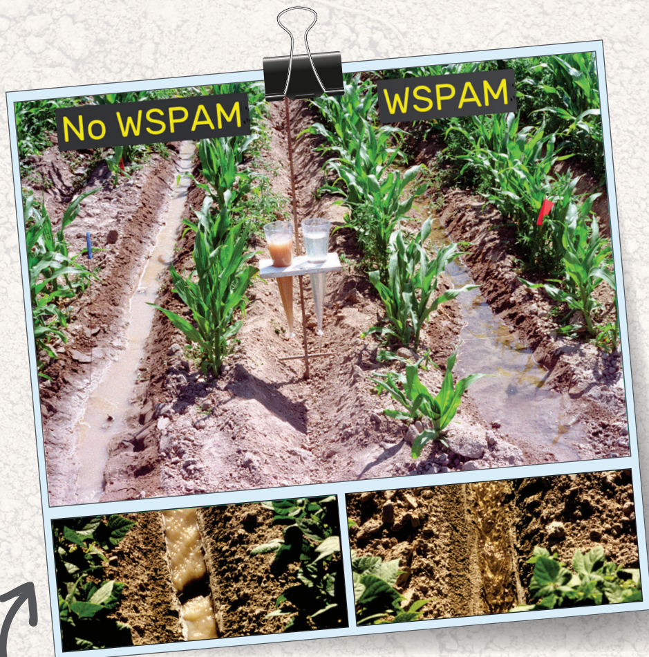
This furrow-irrigated field in southern Idaho has soils with low organic matter and high volcanic ash fractions, which are highly susceptible to erosion. The furrow stream on the left was untreated and shows sediment load and head-cut erosion (lower left). The furrow stream on the right was treated with 10 mg/L water-soluble anionic polyacrylamide (WSPAM) during stream advance.
