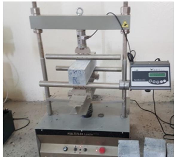
Fig. 7. Flexural test of the SCC prisms.
