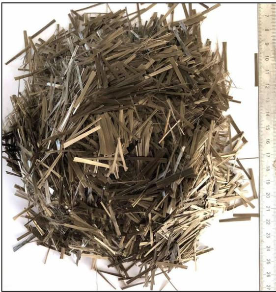
Fig. 2. Basalt fibres used in this study.
