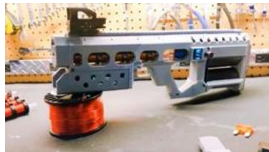
Figure 2-18EMG-01A Coil gun (Nardi 2018)
