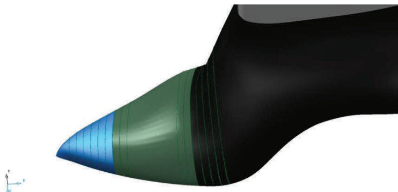
Figure 5. Surface Distortion during Blending by the cross sections due to a Significant Change in Surface Curvature
