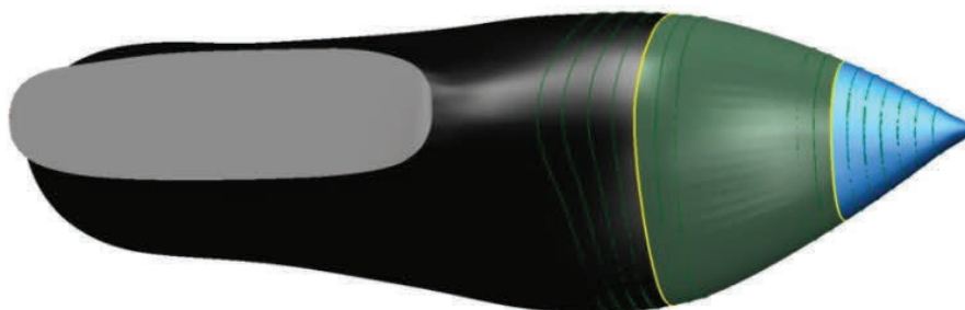
Figure 4. Using the Blending by Cross-Sections Feature for Designing the New Last Shape
