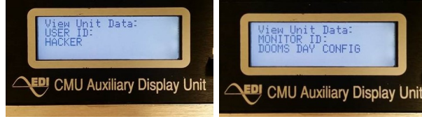
Figure 28: CMU-212 display unit showing the Datakey configuration for USER ID and MONITOR ID which was written using the home-made Arduino Datakey writer to allow for full-permissive configuration.
