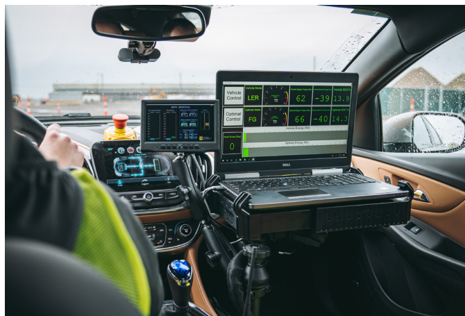
Figure 3-23. In-vehicle engineer's station for conducting real-time tests of the NMPC PTC.
