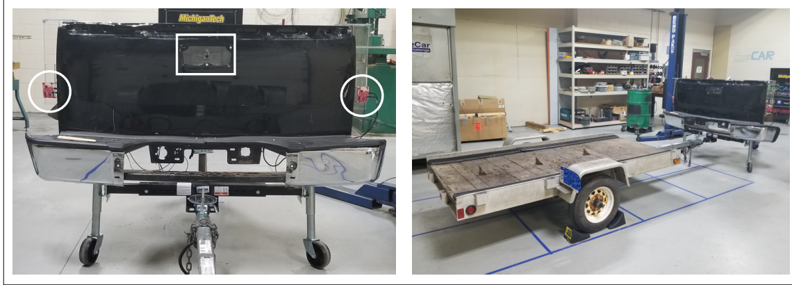
Figure 5.2: Left: The experimental apparatus (truck mock-up) used for radar data collection. Each of the two radars (encircled) is installed on a plexiglass. A protractor , locked to the top of each plexiglass, provides the ground truth of the rotation angle which will be estimated. A rear gate camera (in square bounds) was also installed on the mock-up for visualization of the procedure, it was not used for the calibration. Right: A calibration scenario where corner reflectors were placed on a trailer attached to the truck.
