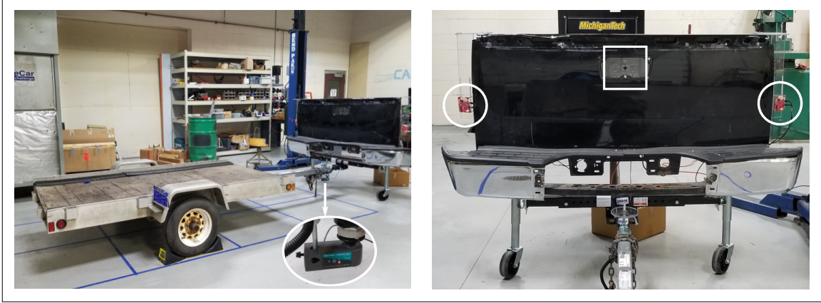
Figure 3.2: Left: The experimental apparatus consists of a trailer coupled with a truck mock-up. The inset image shows a Vernier rotary motion sensor installed on the hitch ball to read the ground truth, it was not used for the estimation. Right: The driver and passenger radars (encircled) installed on the sides of the truck mock-up. A rear gate camera (shown in square bounds) was also installed on the mock-up for trailer visualization, it was not used for the estimation.
