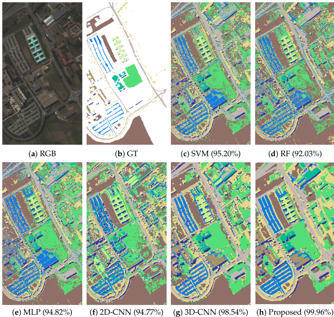
Figure 4. Classification maps for the University of Pavia (UP) dataset. The first image (a) represents a simulated RGB composition of the scene. The second one (b) contains the ground-truth classification map. Finally, images from (c–h) provide the classification maps corresponding to Table 4.
