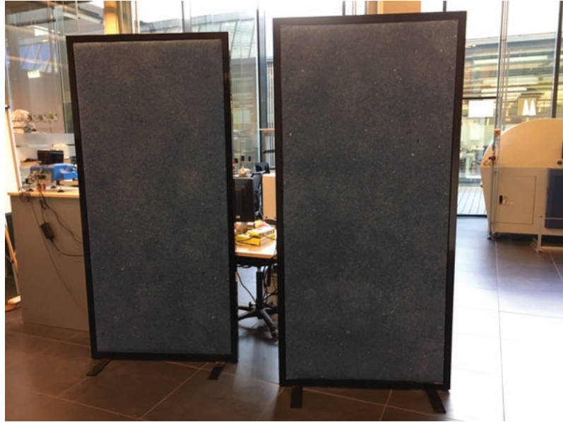
Figure 7.4 Panels from recycled KLM uniforms
