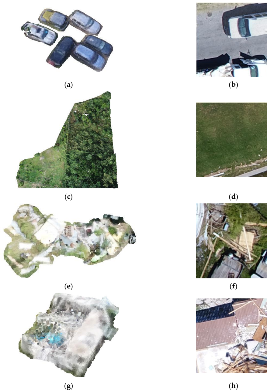
Figure 5. Examples of instances existed from all datasets: (a,b) vehicles, (c,d) terrain, (e,f) debris field, and (g,h) completely damaged structure.
